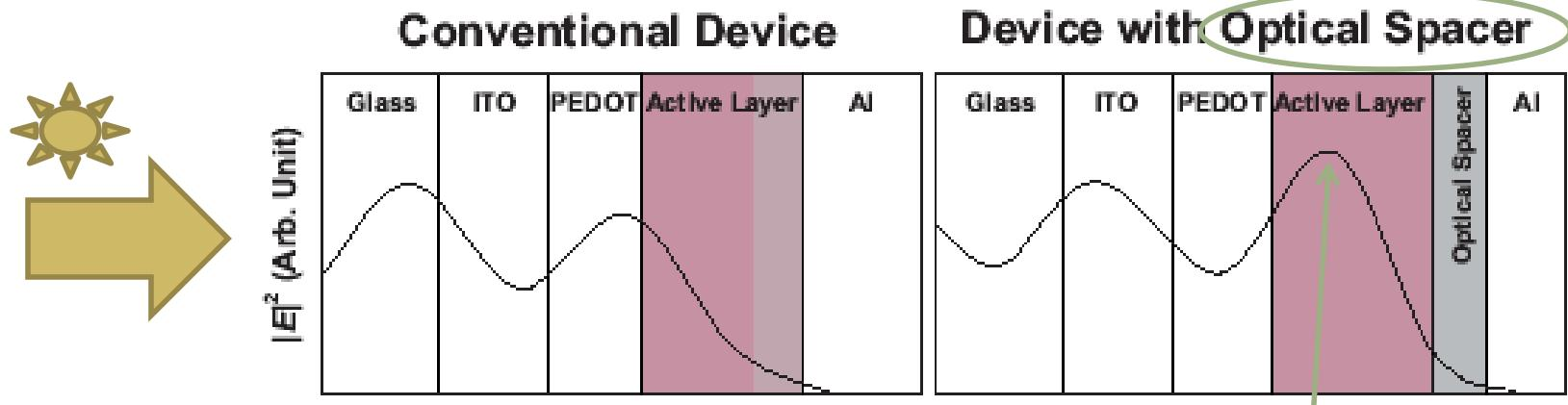
**Maximum of the stationary optical field inside the active region**
