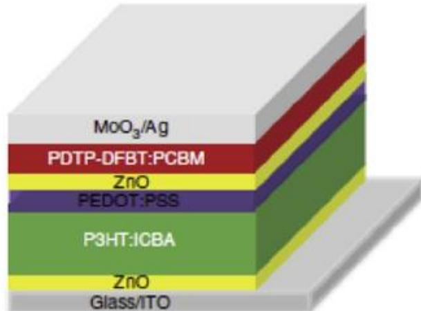
Equivalent  $V_{oc}$ = sum of single cells  $V_{oc}$
