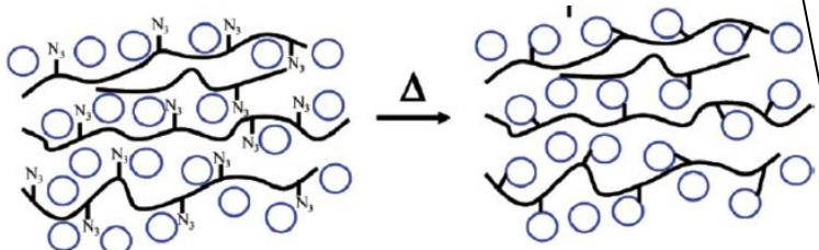
D-to-A linking after deposition
