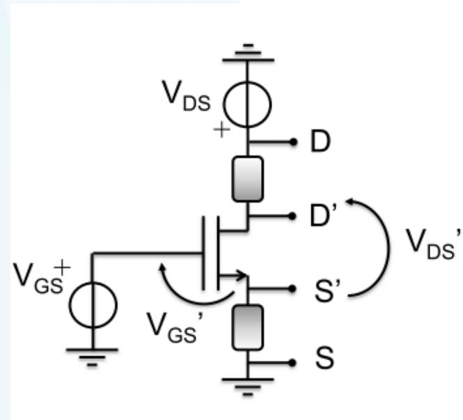
$$\mu_{app} \approx \mu_0 \left( 1 - \left( \frac{\mu_0 C_i W R_C V_{od}}{L + \mu_0 C_i W R_C V_{od}} \right)^2 \right)$$
