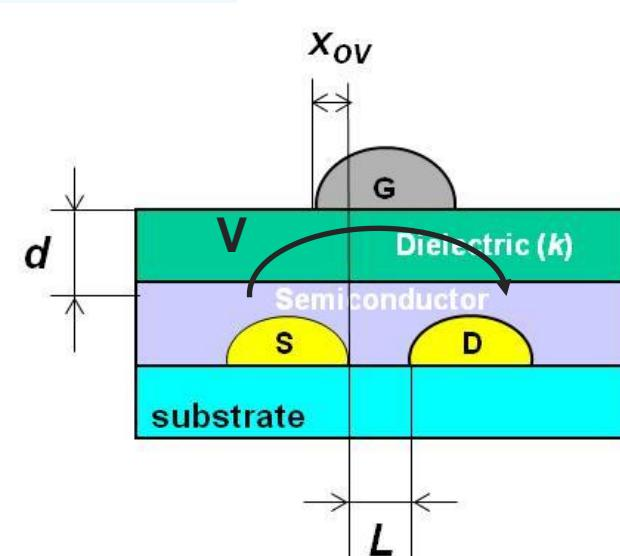
$$\begin{aligned} L &= 10 \mu\text{m} \\ \mu &= 1 \text{ cm}^2/\text{Vs} \\ f_{cut-off} &\approx 400 \text{ kHz} @ 10\text{V} \\ &\approx 2 \text{ MHz} @ 50\text{V} \end{aligned}$$
