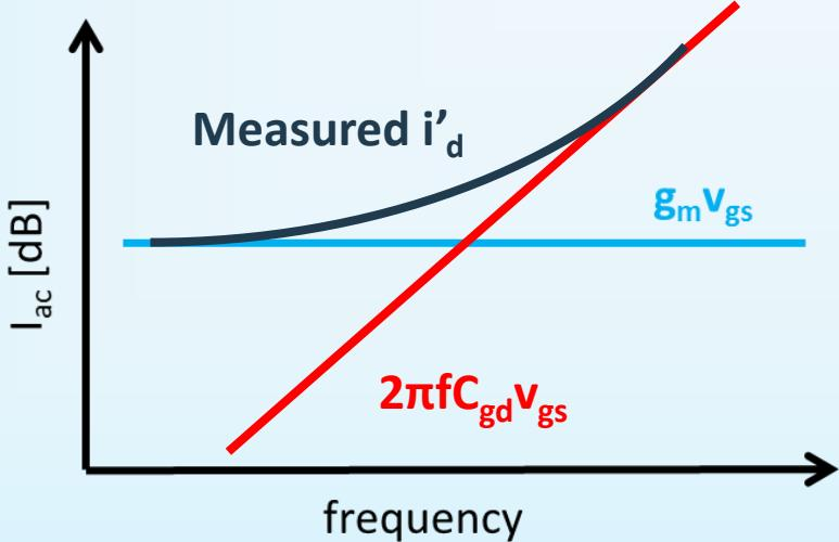
$$i_d' = i_d - i_{cgd} = g_m v_{gs} - j 2\pi f C_{gd} v_{gs}$$
