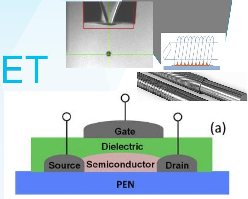
$L = 46 \mu\text{m}$ ,  $W = 1180 \mu\text{m}$ , dielectric thickness = 700 nm,  $V_g = V_d = 40 \text{ V}$
